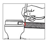
Step 3. Important—Mark position around hose at rear of socket with a grease pencil, paint or tape.
